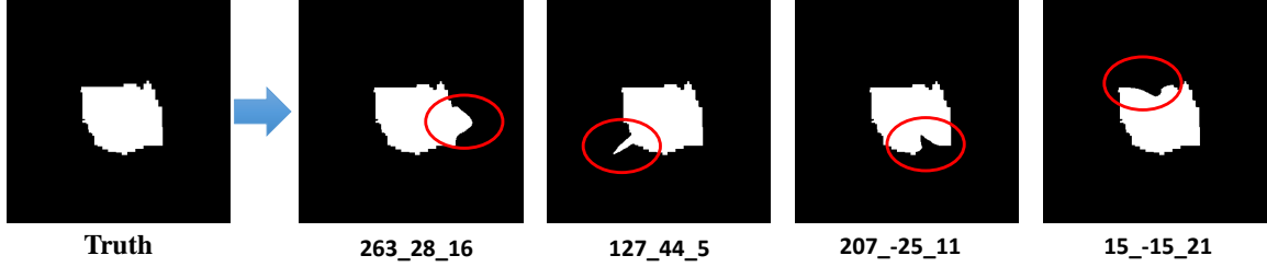
Figure 6. Examples of spiculation error, where emulated boundary spiculation are highlighted by red circles. The three parameters under each emulation from left to right are the center ( c ), height ( h ), and width ( w ). The unit is the pixel. The height can be a positive or negative value to synthesize convex or concave spiculation.
